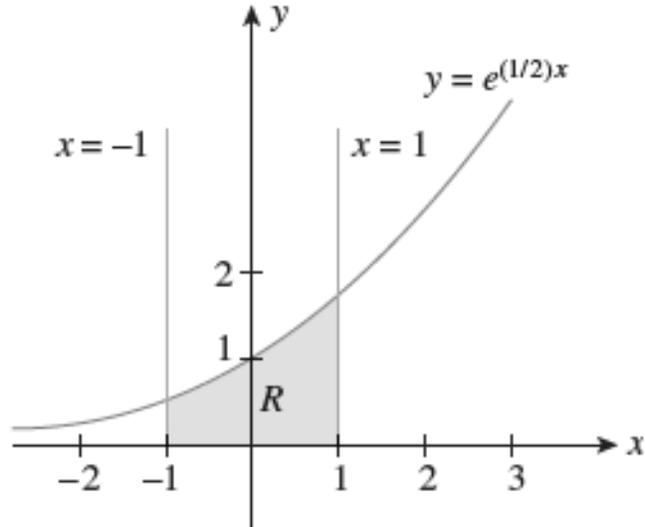
$$R = \int_{-1}^1 e^{x/2} dx = \int_{-1}^1 e^{0,5x} dx \quad \text{por sustitución } \rightarrow t = 0,5x \quad dt = 0,5dx \quad 2dt = dx$$
